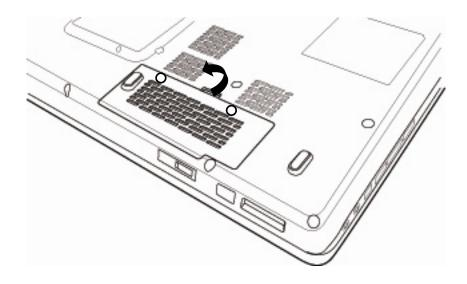
Figure 4-9 Remove Wireless LAN card cover
